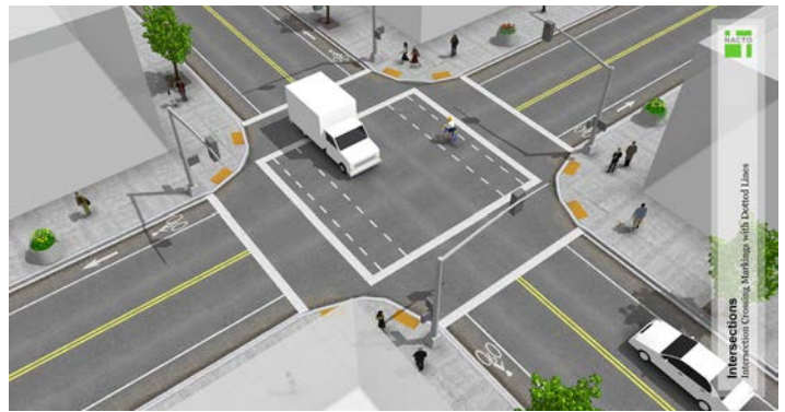
Figure 13: Intersection Crossing Markings
