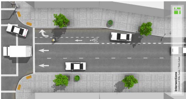
Figure 12: Combined Bike Lane / Turn Lane
