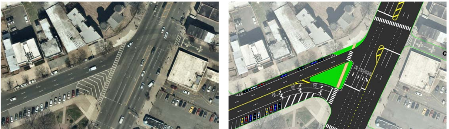
Figure 34: Existing and Recommended alignment of Intersection
